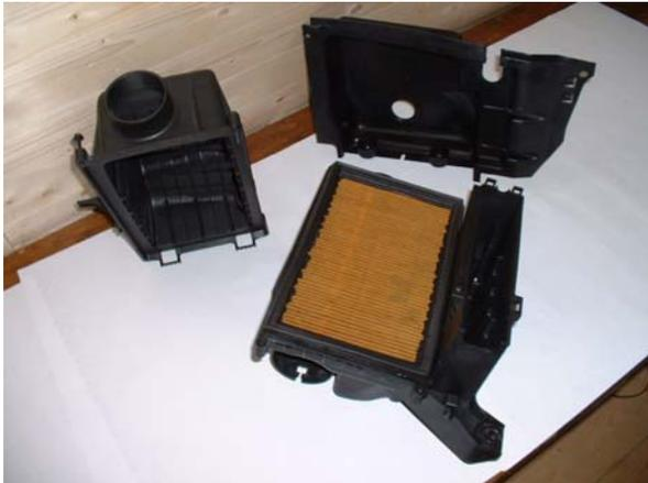
Having done this, open the air filter box, remove the paper filter element and the rubber sealing from the back.
