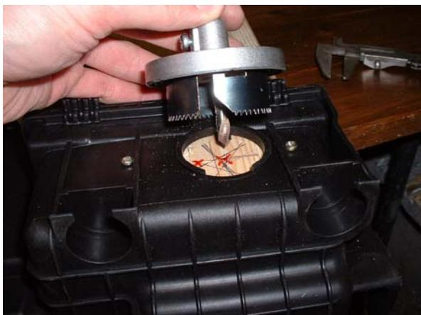
Mark the middle of the hole and put a mark at the same height 14 mm to the left of it. Drill small holes for guidance first, then use a core bit with a diameter of 50 mm and drill very gently with slow speed through the air filter box-wall. Drill once in the middle to enlarge the existing hole and
