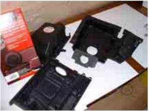
Close the supporting holes you drilled before with some glue. Clean the area for sealing on the partition cowl with pure alcohol to remove any dust, fat or any fingerprints.
