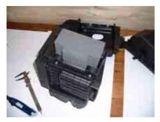
Release the box from the foam block and make some adjusting cuttings make it fits perfectly. Ensure that the diameter in the foam block is not smaller than in the air filter box and partition cowl.
