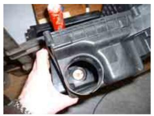
Drill gently two times through the cowl as done before through the air filter box by using the holes in the wooden board as guidance.
