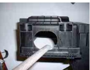
second one is located on right hand side. This is correct as we are looking at the front of the partition cowl, whereas we were looking at the of the lower part of the air filter box previously. Ensure that the wholes for guidance are in parallel to the lower end of the cowl.
