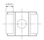
For reflow soldering (propose)
