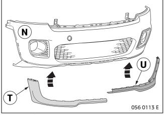
Insert front right spoiler **T** and front left spoiler **U** on the underside of front bumper section **N** and click into place.
