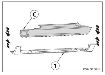
Place upper sill trim **C** on the two previously connected components (1) and click into place.
