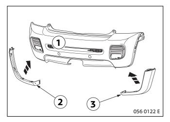
Put the extensions complete with the bulkhead partitions (2) and (3) onto the bumper section (1) from the left and right respectively and click into place.
