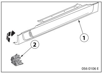
Insert complete sill air inlet (2) into the recessed opening from the back of the sill trim (1) and click into place.
