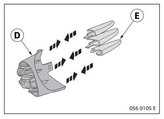
Insert air inlet inserts  ${\bf E}$  into the sill air inlet mounting support  ${\bf D}$ .
