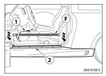
Remove the protective film from the adhesive pad (1) on the bottom of door cutout trim **F**.
