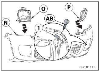
Insert fog light trim **O** and fog light trim **P** in front bumper section **N** and lock into place.
