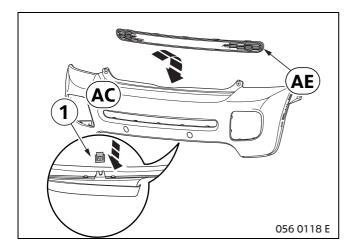
Insert air outlet grille **AE** in bumper trim **AC** from the inside and click into place.
