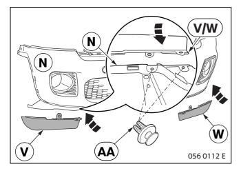
Place ram-air lip **V** and ram-air lip **W** on the bottom of front bumper section **N** and connect with expander rivet **AA**.
