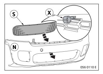
Insert air inlet grille **S** in the front bumper panel **N** and lock into place.
