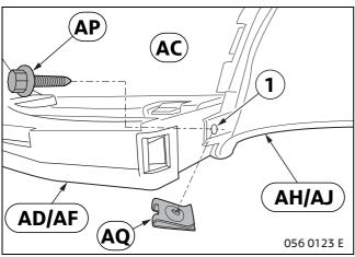
View shows the inside of bumper section **AC**. Make the connection between **AD/AF** and bumper trim **AH/AJ** as follows:
