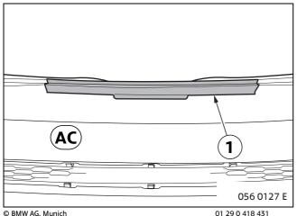
Remove guide rail (1) from series bumper and assemble on retrofit bumper **AC**.
