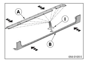
Place adapter fixture **A** on lower sill trim **B**. Insert and lock expander rivets **I** in the holes provided.
