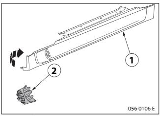
Insert complete sill air inlet (2) into the recessed opening from the back of the sill trim (1) and click into place.
