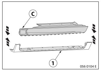
Place upper sill trim **C** onto the two previously connected components (1) and click into place.
