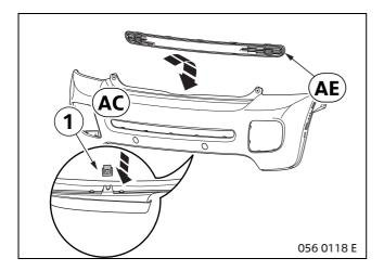
Insert air outlet grille **AE** in bumper section **AC** from the inside and click into place.
