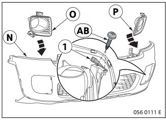
Insert fog light trim **O** and fog light trim **P** in front bumper section **N** and lock into place.
