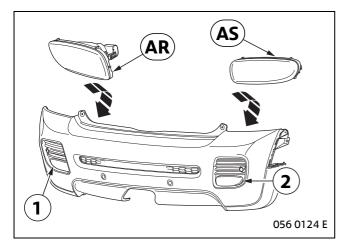
Clip rear fog lights **AR/AS** into left/right air outlet grille (1/2) from the inside.
