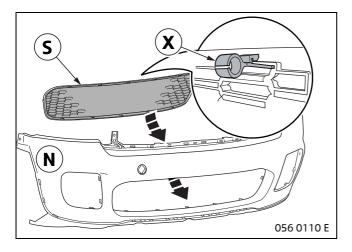
Insert air inlet grille **S** in the front bumper section **N** and lock into place.
