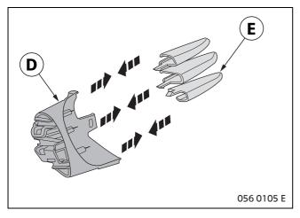
Insert air inlet inserts **E** into the sill air inlet mounting bracket **D**.
