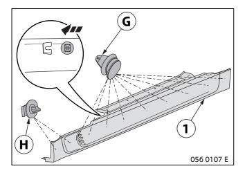
Push white clip **H** and black clip **G** into the retaining grooves provided on the back of the sill trim (1).
