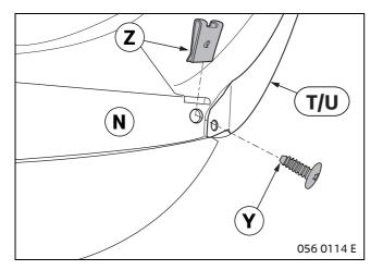
Insert sheet metal nut **Z** in the locating plate on bumper **N**. Attach spoiler **T/U** to the bumper with self-tapping screw **Y**.
