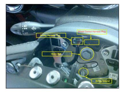
6. This step is only necessary if you have steering wheel controls. Remove 4 #20 Torx screws holding on the airbag retaining plate so that you can remove steering wheel control harness to move to the new steering wheel. (You may want to do this while the steering wheel is still secured on the steering shaft but you can do it once the wheel is removed.) The wheel can now be removed by sliding the wheel off the steering shaft.
