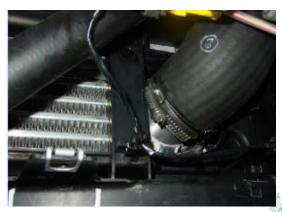
11. At the front of the intercooler, remove the x2 T25 torx screws securing the intercooler to the vehicle.
