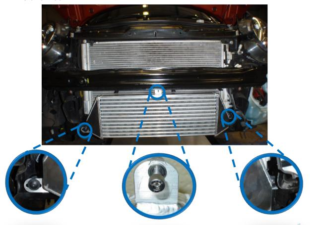
It is not necessary to remove the crash bar to drill the hole for the intercooler, however if you believe you would find it easier you may do so. To remove the crash bar there are x3 13mm nuts at either side that are visible looking from the front of the vehicle. There are x2 lower 13mm bolts visible from the rear of the front panel. The front panel is also attached on the lower edge each side with a T25 torx screw.
