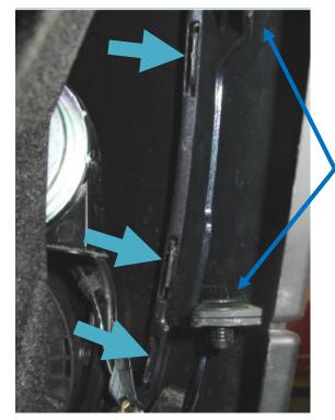
3. Now the wheel arch liner is loose it is possible to access and remove the T25 torx screw that secures the
