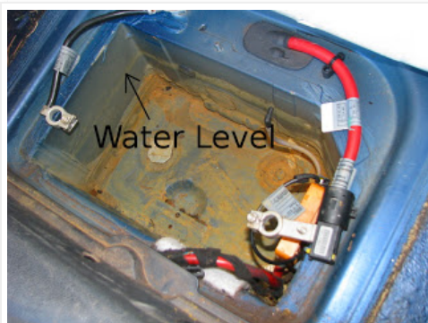
Rust and mud spreading from the screw holes
