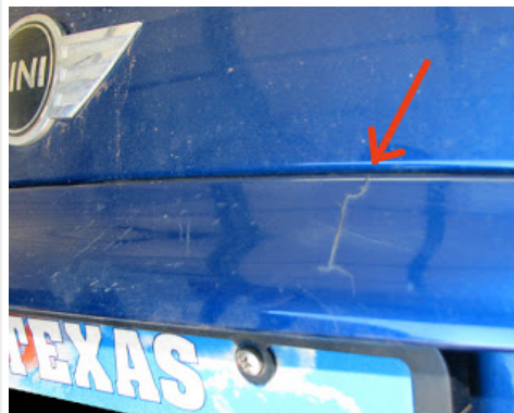
Even a small crack can cause the seal to fail and water to enter the hatch.
