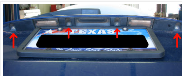
Installation and removal only involves these four screws
