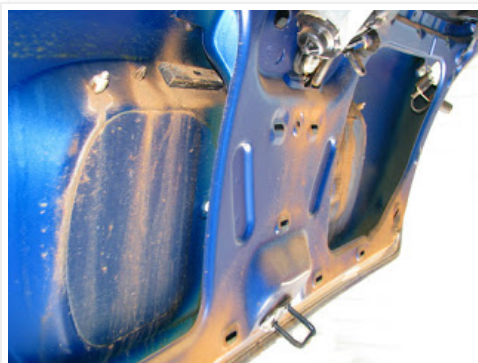
Rust and mud spreading from the screw holes
