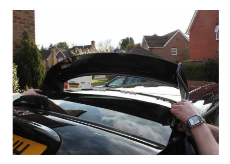
Next insert two M6 stainless steel bolts through the spoiler sides into the riv-nuts in the boot and screw them in using a 4mm Allen key
