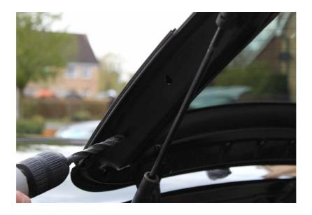
Screw the riv-nut on to the riv-nut tool (not supplied), then place the riv-nut into the drilled hole and squeeze the riv-nut tool to lock the riv-nut in place.
