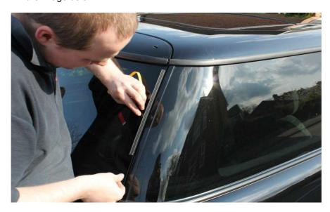
Next place a spoiler side on each side of the boot lid, at the desired height. Mark the two fixing holes with a marker, so that you will know where to drill.
