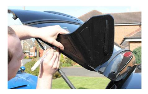
Next remove the spoiler side to reveal the two holes that you need to drill
