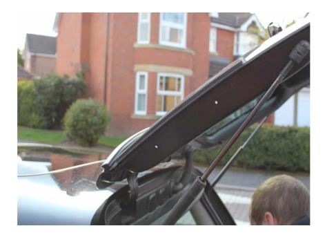
Using the supplied 9mm drill bit, drill all four of the pre-marked holes (two on each side of the boot-lid)
