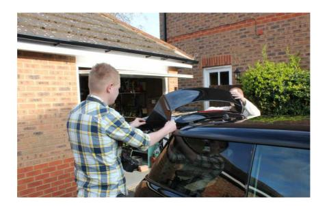
Line up the holes in the spoiler sides with the riv-nuts you installed earlier
