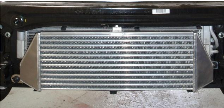
Late 2009 on, upper bracket behind crash bar. Note the crash bar is 10mm lower on the late 2009 cars.
