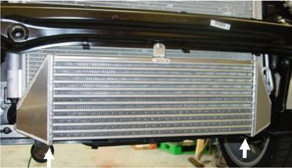
Up to late 2009, upper bracket in front of crash bar
