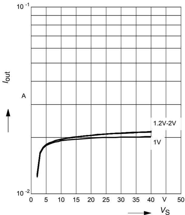
**Output current versus supply voltage**
