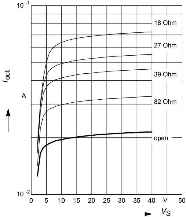
**Supply current versus supply voltage**
