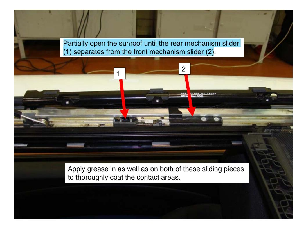
In this channel is a metal rod and plastic bushing which drive the rear mechanism.
