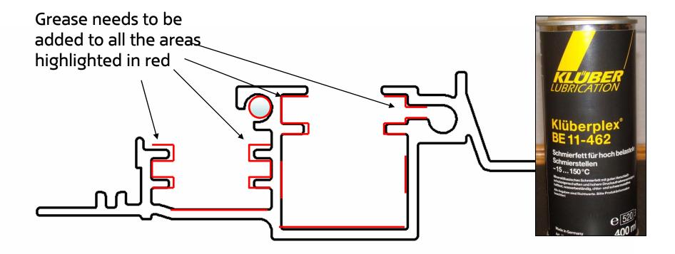
The cross-section to be lubricated should run the entire length of the guide on both the left and right side of the sunroof cassette. The following 2 pages will show this in more detail.
